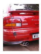
Tail pipe probe can be used with a suitable clamp mounting. The cable may be installed through the rear hatch or window.
